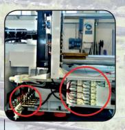
tool and mould making monitoring the cooling circuit from plastic injection moulding machines
