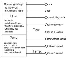
Temperature switch-point adjustment (sensor in contact with medium)
