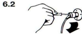
6.2 Turn on normal air flow, wait 3 minutes, adjust pot. (counting the turns) until LED „off“.
